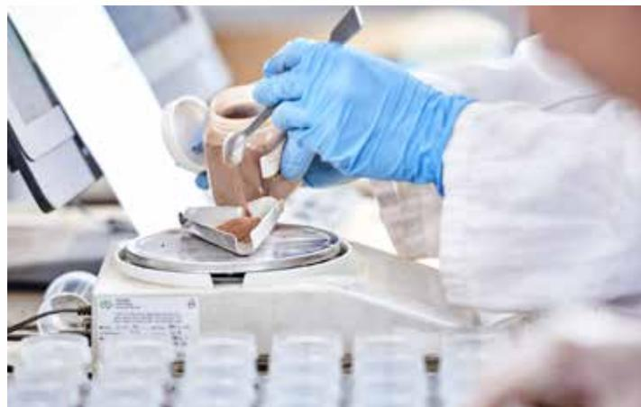
Photo 2: Soil is weighed so that the precise amount needed for the analysis is used.
